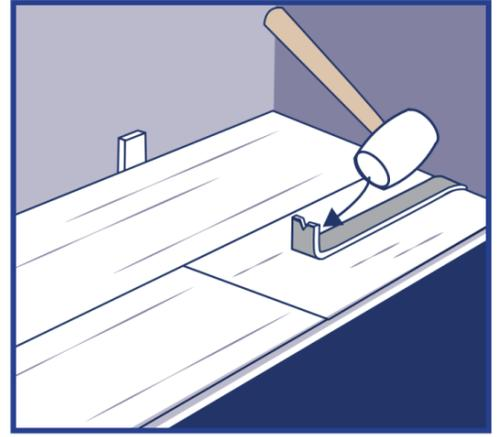
**Step 8: Use hammer and pull bar to lock final piece in row. Insert spacer at end of row. Continue installation to final row.**
